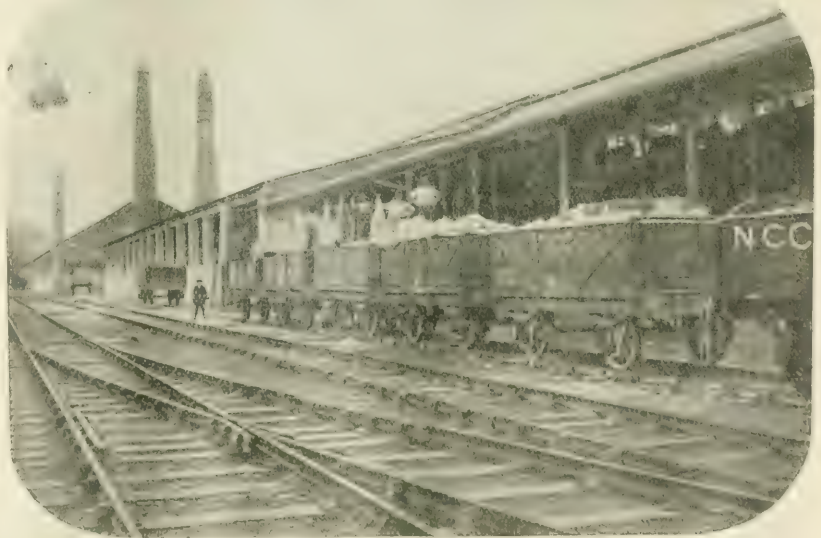
FIG. 13. LOADING CLAY FROM "LINHAYS" INTO RAILWAY TRUCKS. (Photo, English China Clays, Ltd., St. Austell).
